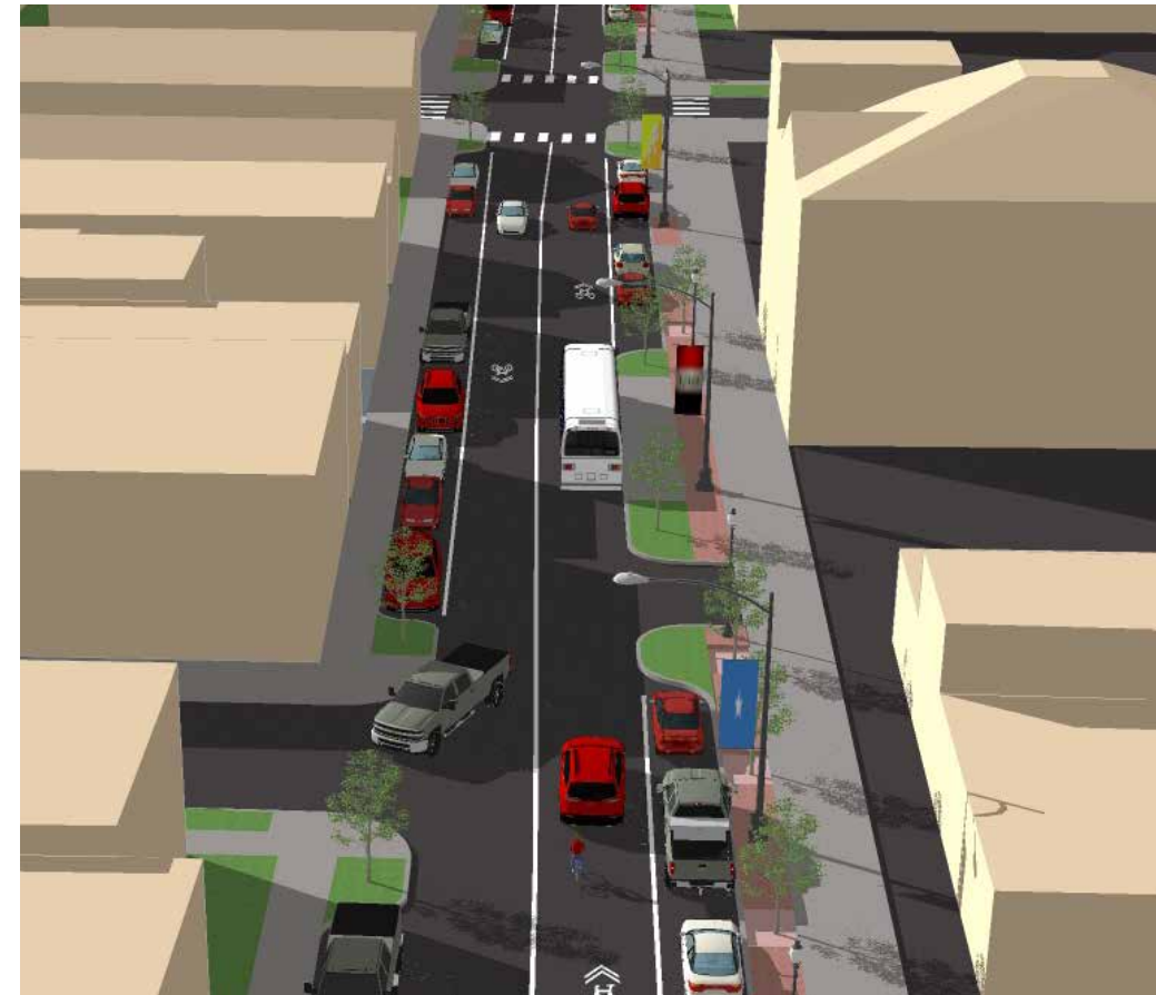
This area can accommodate on-street parking on both sides of the street (W. 44th intersection shown, in distance.) An example of a bus-bulb is shown, in front of the historic Sokol Hall, and public art banners celebrate many of the local residents' nationalities.
