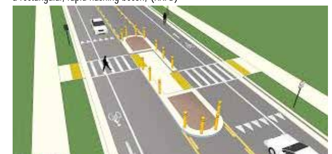
An off-set ladder crosswalks and median pedestrian refuge.
